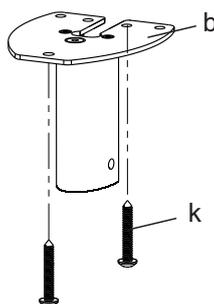
Use a stud finder to locate the stud. It is a good idea to verify where the stud is located with an awl or thin nail. Pre-drill a 50mm deep hole at the stud using a 3.8mm drill bit. Make sure the hole is in the center area of the stud. Use the Ceiling Plate(b) as a template to mark the location of the second hole in the stud. Drill 50mm deep hole using the 3.8mm drill bit in the marked location. Attach the ceiling plate to the ceiling using the 2 pieces Lag Bolts(k).
