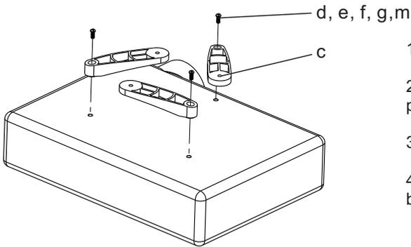
1. Locate the mounting points on the bottom of the projector.
