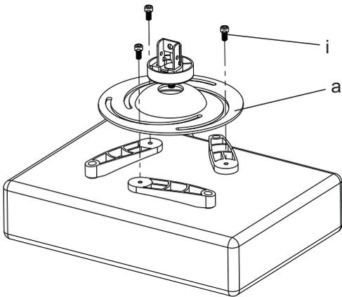
1. Align the Projector Plate(a) to the mounting legs.
