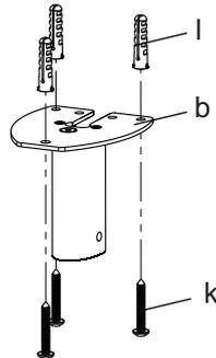
Use the Ceiling Plate(b) as a template to mark 3 hole locations on the ceiling. Pre-Drill these holes with a 8mm masonry bit to at least 50mm in depth. Insert a Concrete Anchor(l) into each of these holes. Make sure the anchor is seated completely flush with the concrete surface even if there is a layer of drywall or other material in front. Attach the ceiling plate to the ceiling using 3 pieces Lag Bolts(k) and 3 pieces Concrete Anchor(l).
