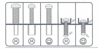
The back of your TV has 4 screw holes in a square or rectangular pattern. This is where the mount will attach to your TV. Suremount provides several sizes and lengths of screws. This guide will help you select the right screws for your TV. You will only use 4 of the provided screws to attach your TV – the rest are not needed.
