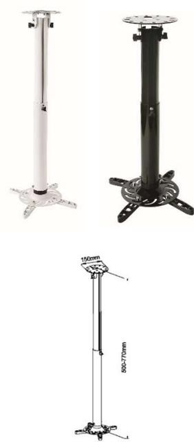
The **SureMount®** SPM03 Extendable projector mount is perfect for most projectors on the market. Weight capacity 15KG and can tilt 30 degrees. Solid extruded aluminum construction adds quality and strength. Has integrated cable management. Fits 95% of all DLP and LCD projectors on the market. Comes with full mounting kit and is available in Black or White. Extension from 500mm – 770mm.
