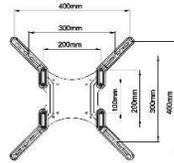
This set of 4 Brackets adds 100MM to each corner 200x200 plate like such as SCL02 and SCL200 becomes 400x400 VESA Pattern. Also useful for TV's with irregular mounting holes.
