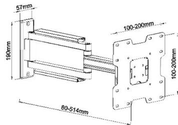
\* Can be extended to (SCL02L) 50” screen and VESA 400x400 with SADAPTOR6 extension bars
