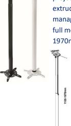
The **SureMount®** SPM05 Extendable projector mount is perfect for most projectors on the market. Weight capacity 15KG and can tilt 30 degrees. Solid extruded aluminum construction adds quality and strength. Has integrated cable management. Fits 95% of all DLP and LCD projectors on the market. Comes with full mounting kit and is available in Black or White. Extension from 1000mm – 1970mm.
