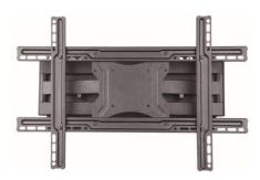
The **SureMount**® SCL06 LCD/LED Dual Cantilever bracket offers full motion movement. Can move left and right 90deg, can also tilt -2 to +12 Degrees. Designed for NZ walls at 635mm with 600mm stud centres. This bracket is ideal for use in a wall recess or when viewing from two positions is desirable. Comes with full mounting kit for both wall and TV fixing.
