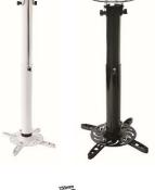
The **SureMount**® SPM03 Extendable projector mount is perfect for most projectors on the market. Weight capacity 15KG and can tilt 30 degrees. Solid extruded aluminum construction adds quality and strength. Has integrated cable management. Fits 95% of all DLP and LCD projectors on the market. Comes with full mounting kit and is available in Black or White. Extension from 500mm - 770mm.
