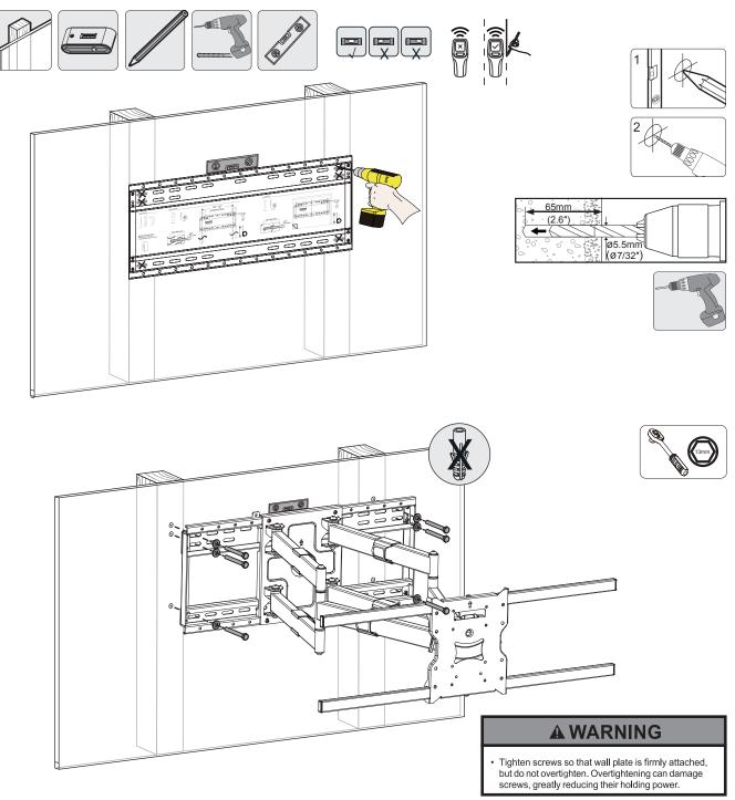
Secure the Wall Plate to the wall with 6 x Lag Bolts (H) and 6 x Washers (H). NOTE: Do not use Wall Anchor (I) for wood stud installation.
