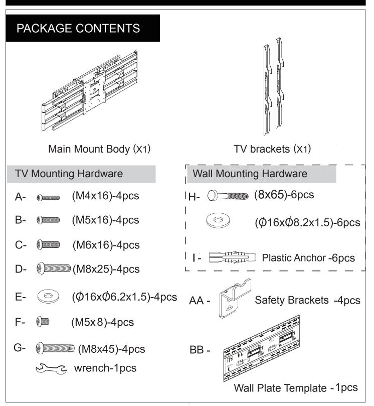
Check carefully to make sure there are no missing or defective parts. Some hardware provided may not be used. Use the correct wall mounting and TV mounting hardware suitable for your installation. CAUTION: DO NOT INSTALL ON DRY WALL ALONE. INSTALL MOUNT ON WOOD STUDS. USER MUST VERIFY THE WALL CAN HOLD THE WEIGHT OF THE TV AND THE TV MOUNT.
