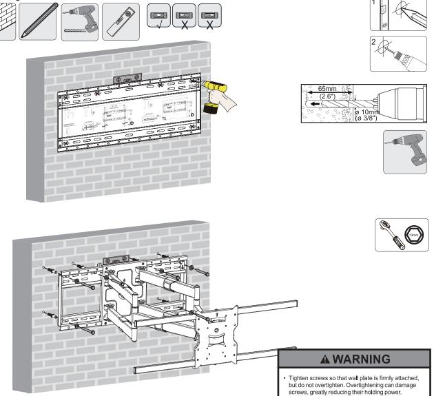
Insert 6 x Wall Anchors (I) into holes. Secure the Wall Plate to the wall with 6 x Lag Bolts (H) and 6 x Washers (H).
