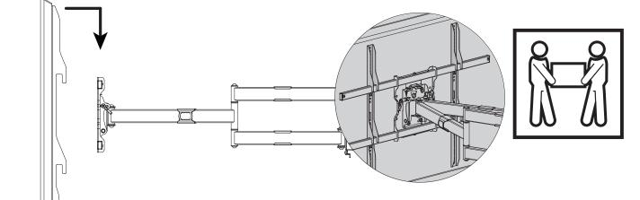
Lift the TV up (two persons recommended) and hang the TV brackets on to the wall mount extension bars.
