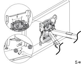
Attaching the TV to the Mount (For Displays With Larger Bolt Hole Patterns) For TVs with larger bolt hole patterns of VESA 300x300,400x200,400x400,600x400, 800x600 mm, use the TV brackets and the extension bars to install the TV to the mount.
