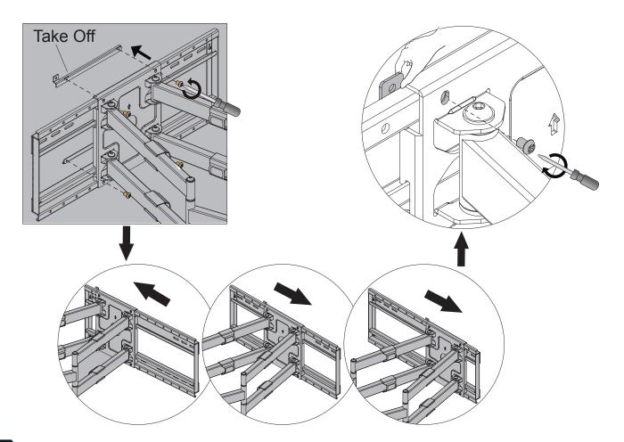
3a. Attaching the TV to the Mount (For Displays With Smaller Bolt Hole Patterns) For TVs with smaller bolt hole patterns of VESA 100x100, 100x200, 200x100 and 200x200mm, the TV can be mounted directly on the plate, without the extension bars.
