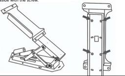
3. Place the lift unit in its desired installation location & mark the hole positions. Drill 10mm holes & insert (A) wall plugs. Screw the lift unit into place using screws supplied (B) into (A) wall plugs.
