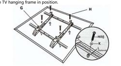
6. Screw (E) the TV hanging frame to the front panel of the TV lift unit using one of the three-hole height positions. The measurements taken in step 4 will help to ascertain the correct holes to use
