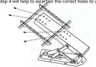
7. Place the lift unit in its desired installation location & mark the hole positions. Drill 10mm holes & insert (A) wall plugs. Screw the lift unit into place using screws supplied (B) into (A) wall plugs.
